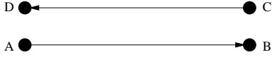
Figure 3: Example that demonstrates that power control alone is not enough to combat the near-far problem in MANETs.
