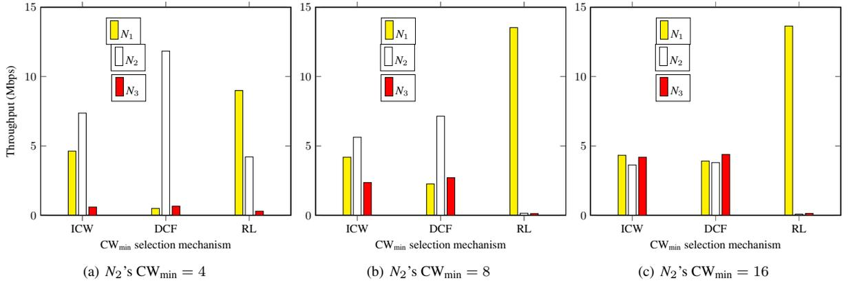
FIGURE 11: Per-node uplink throughput under three mechanisms for setting CW<sub>min</sub> at  $N_1$ , when  $N_2$  sets its CW<sub>min</sub> to (a) 4, (b) 8, and (c) 16.
