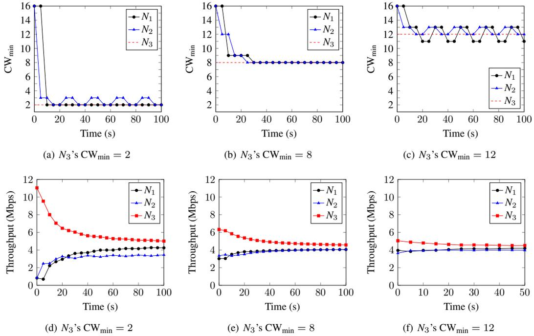
FIGURE 15:  $CW_{\min}$  value of all nodes vs. time, when  $N_3$  is having  $CW_{\min}$  values of (a) 2, (b) 8, and (c) 12, and their respective uplink throughput in (d), (e), and (f), respectively ( $L = 3$ ).
