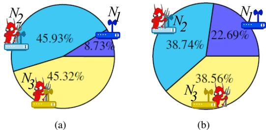
FIGURE 1: Relative per-node throughput for a network of three nodes. Nodes  $N_2$  and  $N_3$  are aggressive with  $CW_{\min}$  set to 4: (a)  $N_1$ 's  $CW_{\min}$  is set to 16, (b)  $N_1$  randomly selects its  $CW_{\min}$  between 2 and 16.
