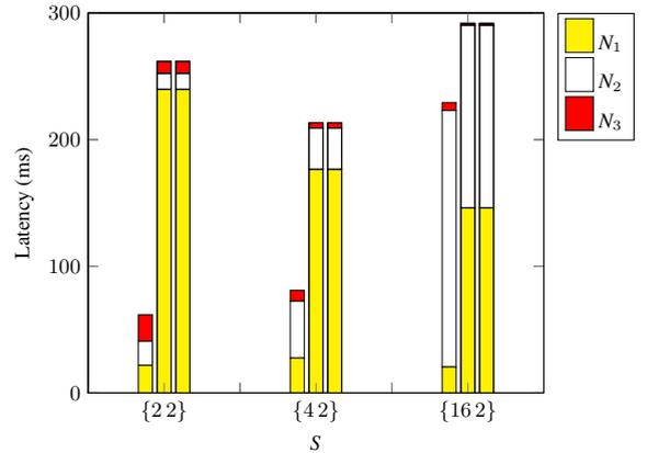
FIGURE 13: Per-frame latency under three mechanisms for setting CW<sub>min</sub> at node  $N_1$  and three different values for  $S$ . “Color only”, “angled lines”, and “dots” patterns represent ICW, DCF, and RL, respectively.
