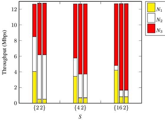
FIGURE 12: Uplink throughput under three mechanisms for setting CW<sub>min</sub> at node  $N_1$  and three different values for  $S$ . “Color only”, “angled lines”, and “dots” patterns represent ICW, DCF, and RL, respectively.
