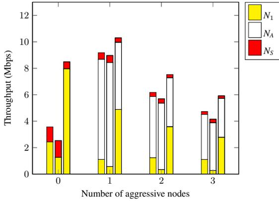
FIGURE 14: Upnlank throughput under three mechanisms for setting  $CW_{\min}$  at node  $N_1$  vs. number of aggressive nodes. “Color only”, “angled lines”, and “dots” patterns represent ICW, DCF, and RL, respectively.
