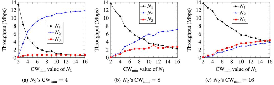
FIGURE 10: Per-node uplink throughput vs.  $N_1$ 's CW<sub>min</sub> when  $N_2$  has a CW<sub>min</sub> value of (a) 4, (b) 8, and (c) 16.
